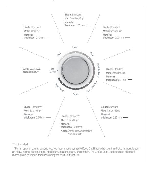
**Tip:** The Smart Set<sup>m</sup> dial has been calibrated to work best with Cricut<sup>m</sup> branded products. If settings either don't cut all the way through the material or the blade is cutting too deeply into your mat, use the half settings located between the material markings on the dial which will increase or decrease the pressure.
